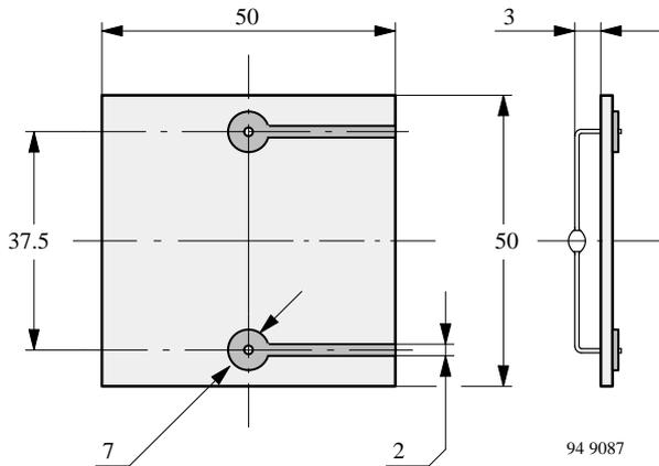
Figure 1. Epoxy glass hard tissue, board thickness 1.5 mm,
